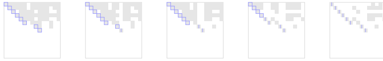
Figure 1.2: Back substitution on the large matrix from figure 1.1. You can see the first few steps, and then a step somewhere in the middle of the calculation, and then the final result. You can see the pivots turn into 1's.
